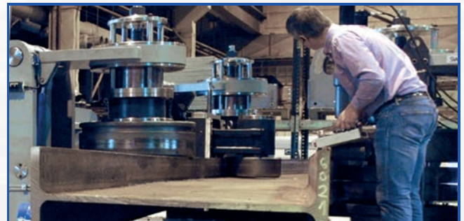
Rolling a HEA800 in a variable geometry Section Bending machine
