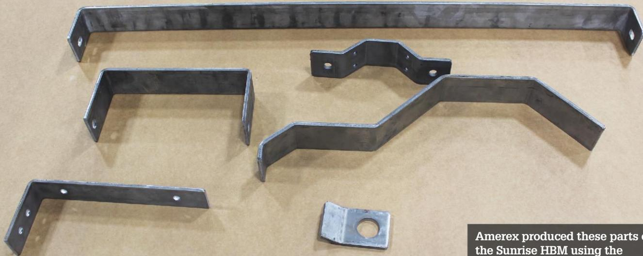
Amerex produced these parts on the Sunrise HBM using the machine's press brake tooling capability.
