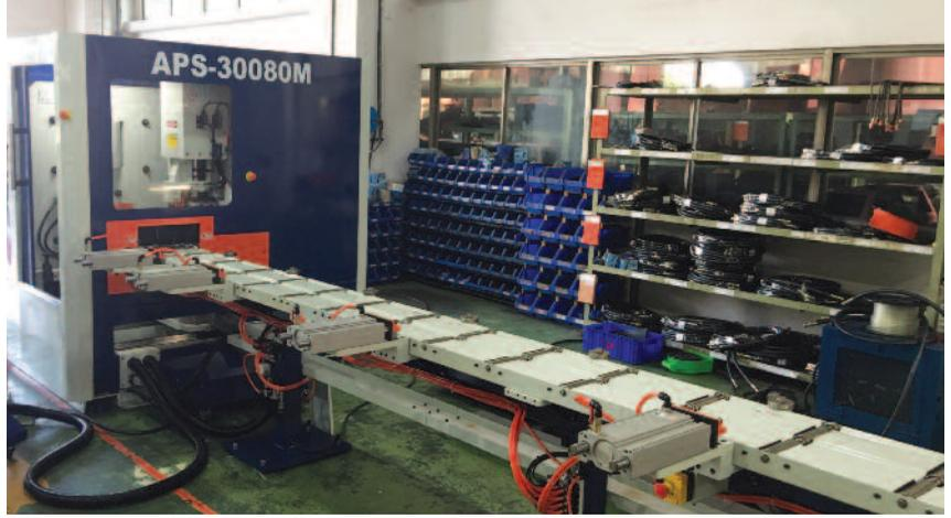
can process materials up to 12 in. wide,  $\frac{3}{4}$ -in. thick and 20-ft. long.
