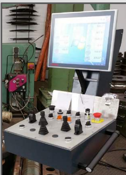
Possibility to use a standard TFT screen to display axis positions in large format that may be seen from a distance if machine is operated through our wireless control unit.
