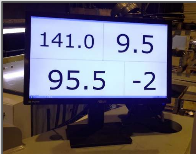
Possibility to use a standard TFT screen to display axis positions in large format that may be seen from a distance if machine is operated through our wireless control unit.
