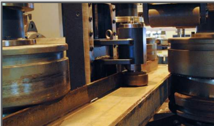
Rolling a C15 x 50# using standard pulling head & universal rolls
