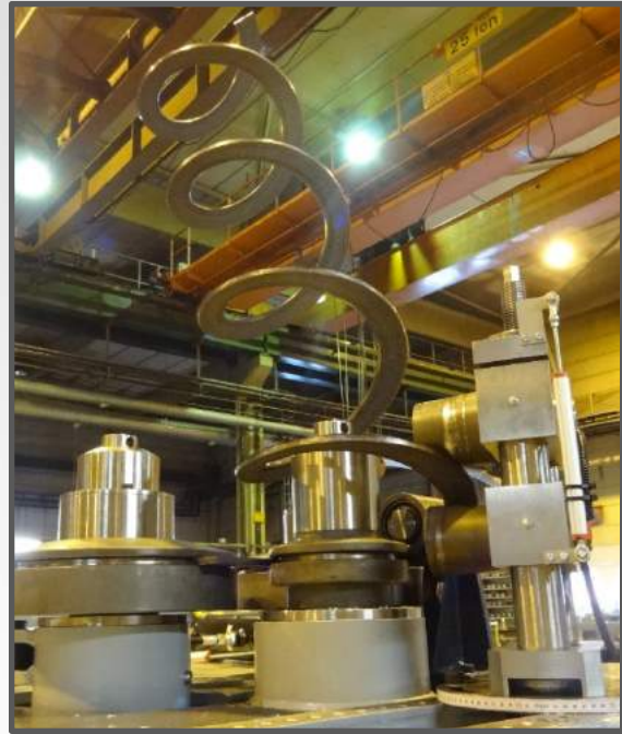
Hydraulic spiraling equipment is used to produce flat bar spirals (“augers”, “flights”) in various dimensions.
