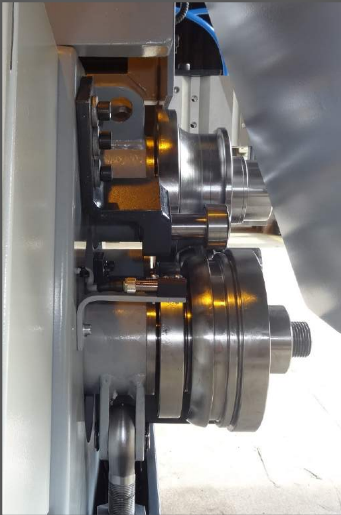
Special rolls & equipment to roll aluminum sections on SB3B-55
